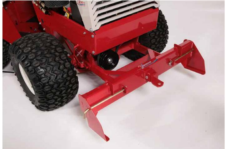
The 2-N-1 fits the front of either 3000 or 4000 series tractor and combines the 2 inch receiver tube for towing with a Front Counter-Weight Bracket capable of holding six 42 lbs (19 kg) weights.
