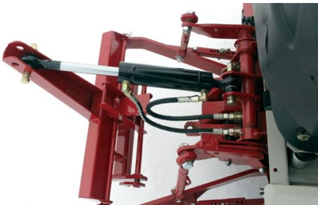
The Hydraulic Top Link is a great accessory to use with the Ventrac Category One 3-Point Hitch option. It allows for fast and easy mounting of attachments when used with the Ventrac 3-N-1 Hitch. (Blades, Slip Scoops, Terra Rake, etc.)
