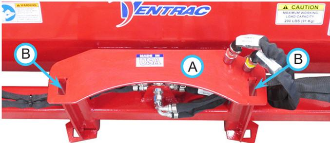
2. Drive forward slowly until the power unit hitch tabs are aligned with the hitch point slots (B) in the snow bucket hitch frame. Raise the power unit hitch to engage the tabs in the hitch point slots. Continue to raise the hitch until the snow bucket is lifted off the ground.
