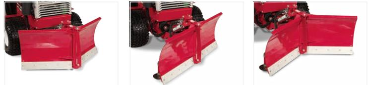
The 55-inch wide Ventrac KV552 V-Blade maximizes efficiency with the ability to quickly change from V-plow to scoop to straight blade, all from the convenience of Ventrac's exclusive S.D.L.A. Control System. With a 48" V width, the KV552 is ideal for walks and areas that larger blades are unable to plow.
