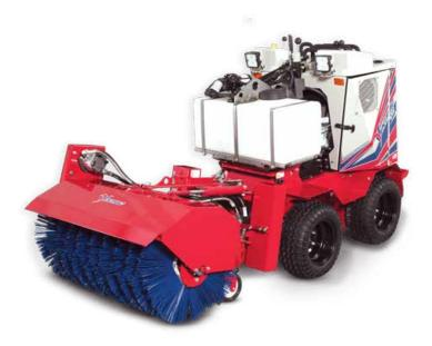
The NJ380 Power Broom for the Ventrac SSV features a working width of 38 inches and an angled width of 35 inches, making it a perfect solution for cleaning snow and debris from sidewalks and walkways.
