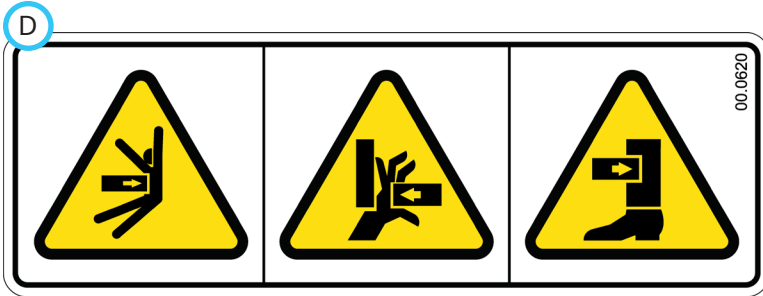
Pinching or crushing hazard.
